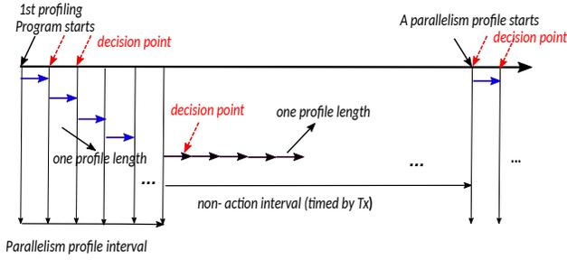
Fig. 2. **Periodical profiling procedure.** At each decision point (marked by dashed red arrow), the actions are taken. Each decision points corresponds to one state of an automaton as in Fig. 3(b) and Fig. 5.
