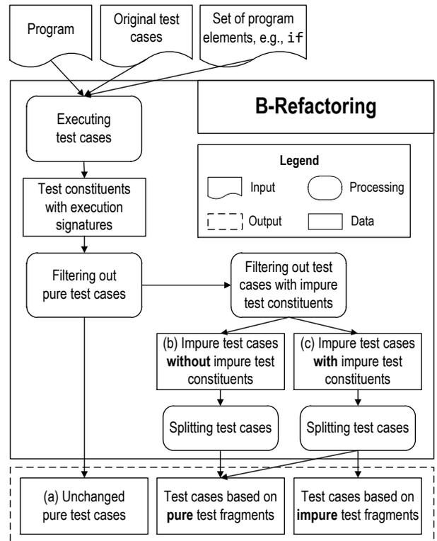
Fig. 2: Conceptual framework of B-Refactoring. This framework takes a program with test cases and a specific set of program elements (e.g., `if` elements) as input; the output is new test cases based on test fragments. The sum of test cases in (a), (b), and (c) equals to the number of original test cases.
