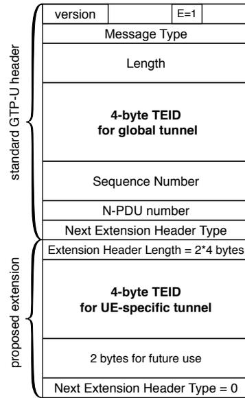
Fig. 7. Extended GTP-U header
