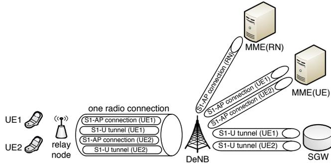
Fig. 2. Tunnels and connections with fixed relays
