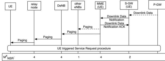
Fig. 6. Network triggered Service Request procedure (NSR)
