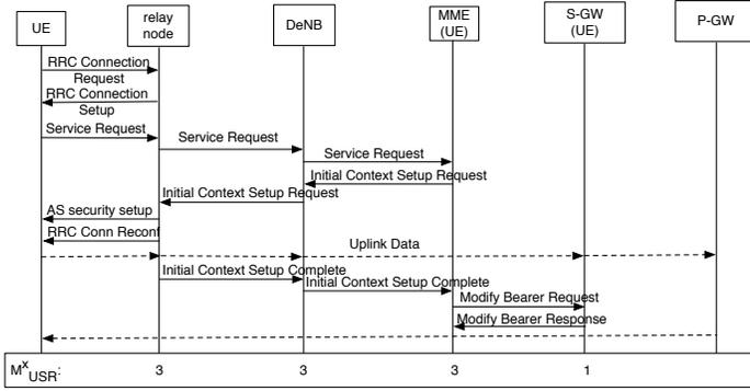
Fig. 5. UE triggered Service Request procedure (USR)
