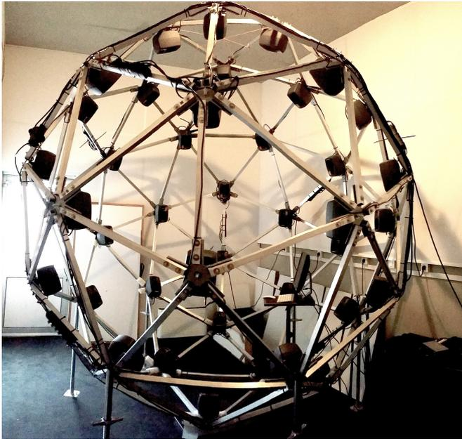
**Figure 1:** Picture of the spherical loudspeaker array.
