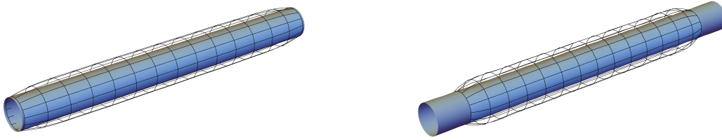
Figure 3: Initial (filled) and deformed (contour lines) shapes of the shell: [left] shell under actual pressure (point A in Fig. 2); [right] shell under radial force (point B in Fig. 2)
