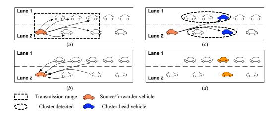
Figure 3: Main phases of SRB technique: (a) RTB transmission, (b) CTB transmission, (c) Cluster detection and CH election, and (d) message propagation.
