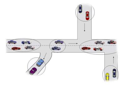
Figure 1: Schematic of several vehicle clusters. Vehicles belonging to the same cluster can communicate each other, while due to gaps among consecutive clusters, no inter-cluster communications are available.
