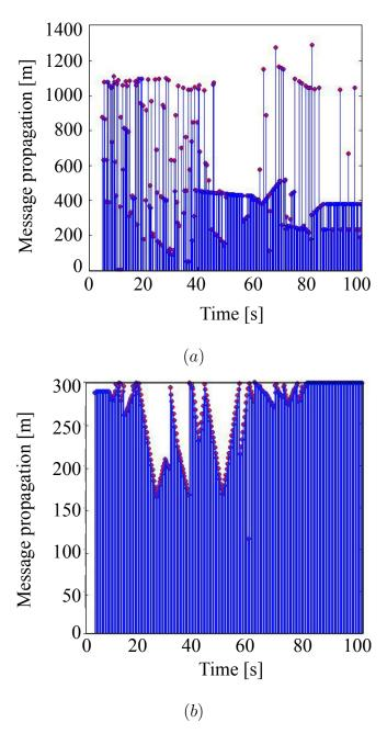
Figure 8: Urban scenario. Average message propagation for (a) SRB technique, and (b) broadcast approach, vs. simulation time.
