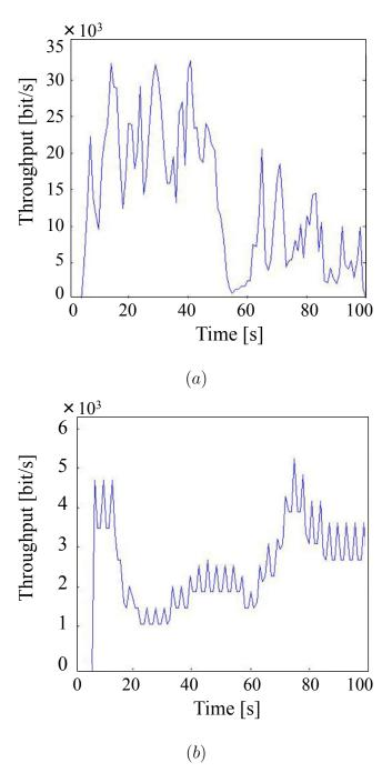
Figure 6: Urban scenario. Average throughput for (a) SRB technique, and (b) broadcast approach, vs. simulation time.
