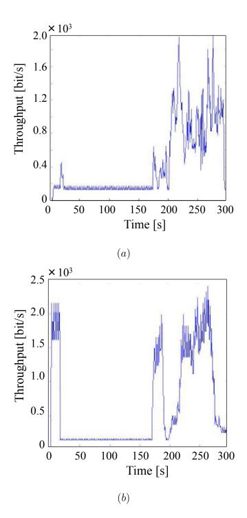
Figure 10: Highway scenario. Average throughput for (a) SRB technique, and (b) broadcast approach, vs. simulation time.
