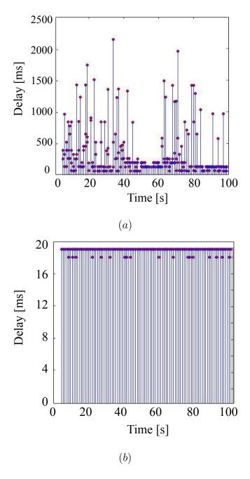
Figure 9: Urban scenario. Average end-to-end delay for (a) SRB technique, and (b) broadcast approach, vs. simulation time.
