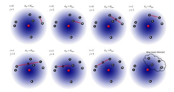
Figure 4: Cluster detection mechanism implemented in SRB technique. From left to right, each vehicle computes the inter-distance among neighbors (i.e.,  $d_{ij}$ ) and compares it to the threshold (i.e.,  $D_{min}$ ), till the cluster is detected.
