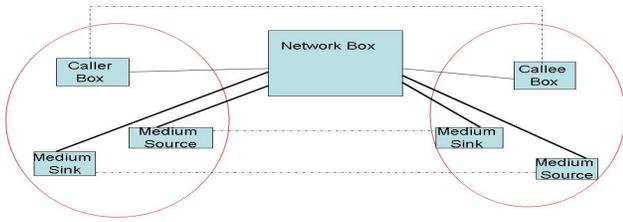
Figure 1: Architecture of the partial session transfer and retrieval. Thick lines show the connectivity established by the network box to medium sources and sinks.
