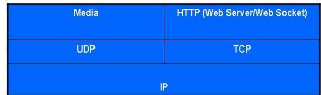
Figure 3: Protocol stack for medium devices.
