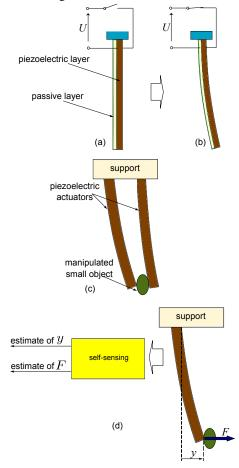
Fig. 1: (a) and (b), principle of a unimorph piezoelectric cantilevered actuator. (b) a microgripper with two piezoelectric cantilevered actuators. (c) simultaneous estimation of the displacement and of the manipulation force by using self-sensing.
