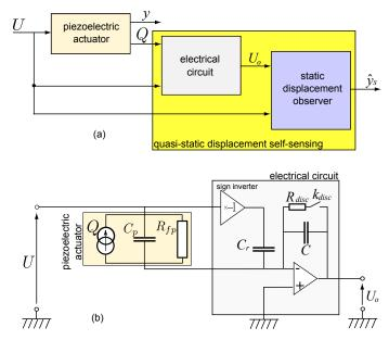
Fig. 2: (a) Principle scheme of the quasi-static displacement self-sensing. (b) the electrical circuit [25].
