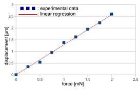
Fig. 8: Steady-state force-displacement characterization used to identify the piezoelectric compliance  $s_p$ .
