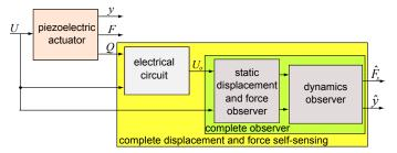
Fig. 4: Principle scheme of the complete displacement and force self-sensing.
