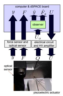
Fig. 7: Setup used for the experimental tests.
