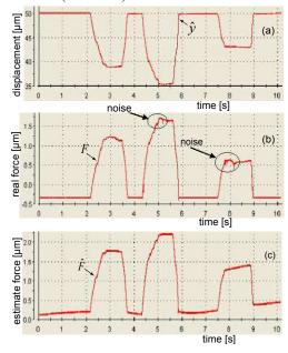
Fig. 15: Experimental result on tracking of a reference displacement  $y_r$  with  $F \neq 0$  (the actuator is in contact with an object). (a): the estimate displacement  $\hat{y}$ . (b): the measured (real) force F. (c): the estimate force from the self-sensing measurement technique.
