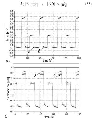
Fig. 10: Experimental results. (a): force F measured by an external force sensor and estimate force  $\hat{F}$  from the selfsensing. (b): displacement y measured by an external optical sensor and estimate displacement  $\hat{y}$  from the self-sensing.
