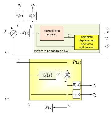
Fig. 12: (a): the closed-loop scheme augmented with the weightings. (b): the corresponding standard scheme.
