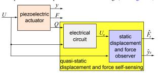
Fig. 3: Principle scheme of the quasi-static displacement and force self-sensing.
