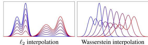
**Figure 2:** Comparison between Euclidean (left) and Optimal Transport (right) barycenters between two densities, one being a translated and scaled version of the other. Colors encode the progression of the interpolation. The Euclidean interpolation results in mixtures of the two initial densities, while Optimal Transport results in a progressive translation and scaling.
