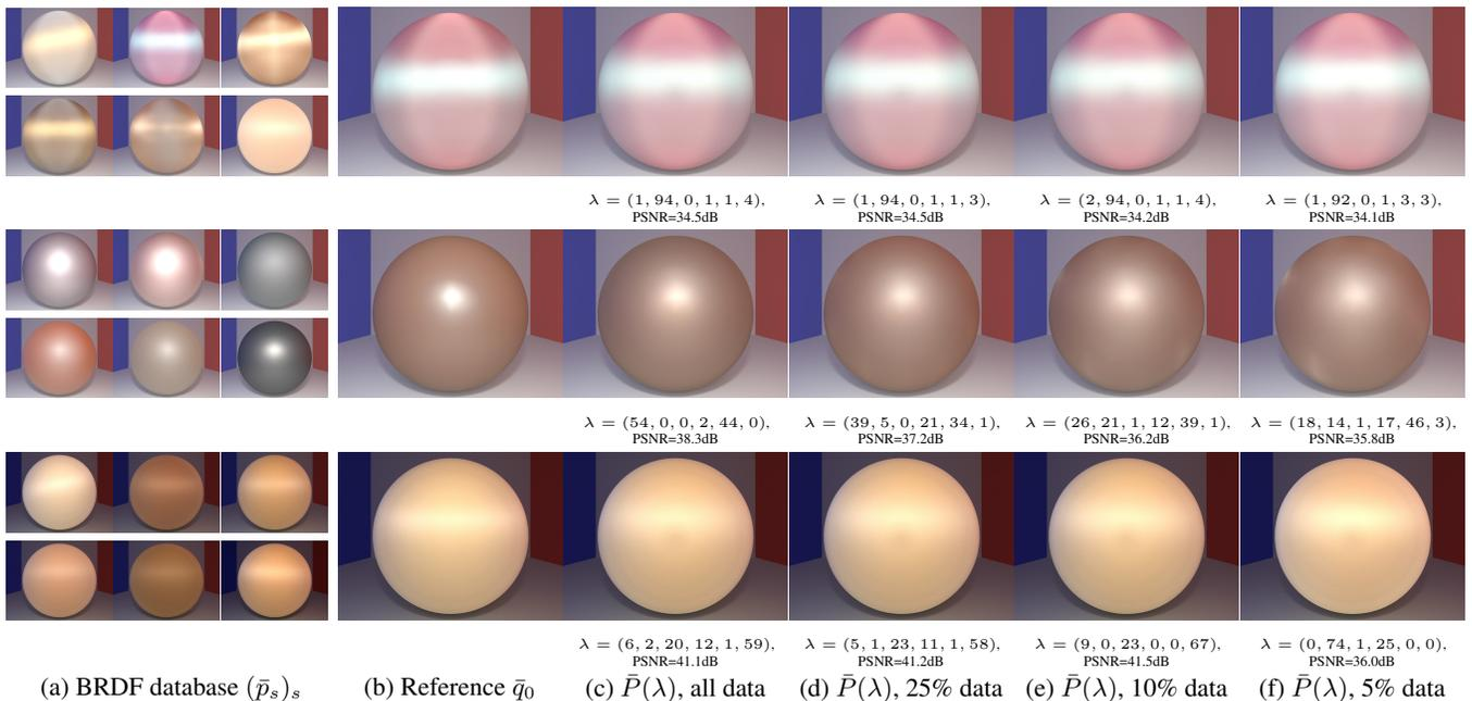
**Figure 6:** We fit a measured anisotropic BRDF  $\bar{q}$  (b) using a basis of  $S = 6$  measured BRDFs  $(\bar{p}_s)_{s=1}^S$  (a). We obtain an approximation  $\bar{P}(\lambda)$  (c) that remains robust when decimating measurements prior to the fitting (d,e,f). Reported  $\lambda$  are normalized so that  $\sum_s \lambda_s = 100$ , and PSNR values computed on BRDFs.
