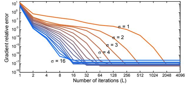
**Figure 5:** Gradient accuracy compared to finite differentiation. We use the  $S = 3$  2D histograms of Fig. 4 (downsampled to  $N = 64 \times 64$ ), and vary the number of iterations  $L$  and  $\gamma = 2\sigma^2$ .
