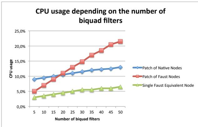
Figure 9: Comparison of performances for multiple biquads
