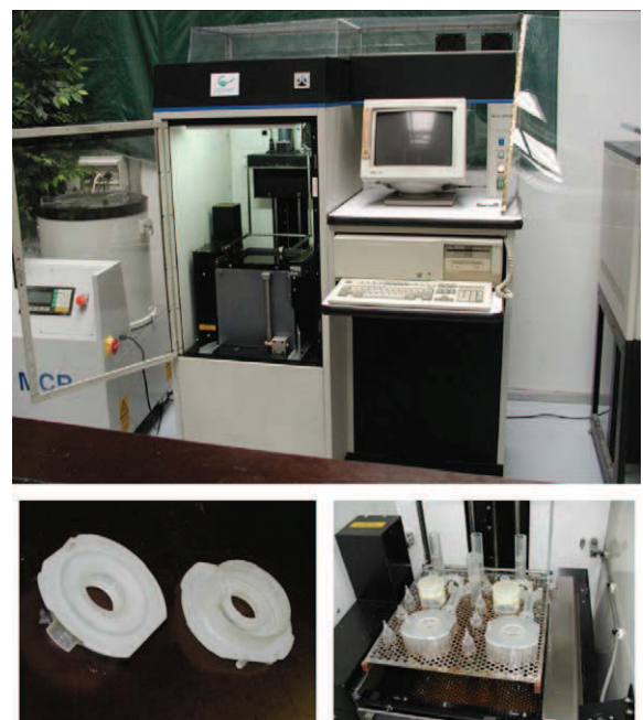
Fig. 12. Stereolithography machine and return ring patterns.
