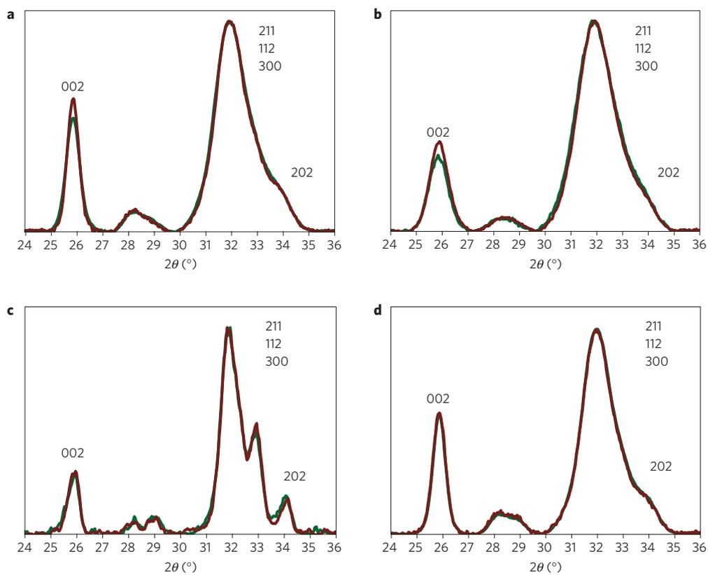
**Figure 4 | Orientation of biomimetic HA platelets. a-d**, 1D radial average of the WAXS patterns for dry (green) and H<sub>2</sub>O wet (red) CHA (**a**), CHA-SBF (**b**), HCA (**c**) and CHA-200 (**d**) powders.
