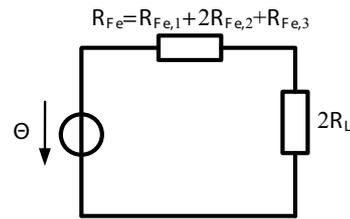
Figure 2: Equivalent circuit diagram
