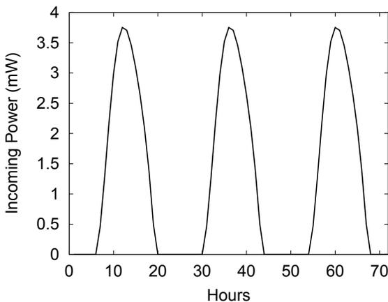
Fig. 4: Incoming power during three sunny days.
