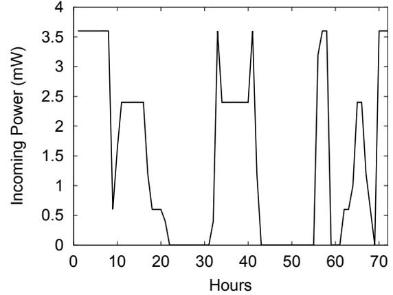
Fig. 8: Incoming power during three unpredictable days.
