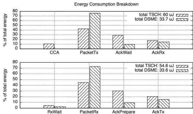
Figure 5. Energy consumption breakdown for different phases
