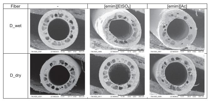
**Table 5**Scanning electron microscopy images of the C fibers with ionic liquid immobilized.
