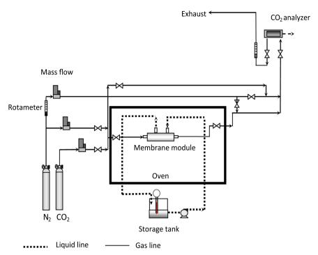
Fig. 2. Experimental setup for CO<sub>2</sub> gas capture.
