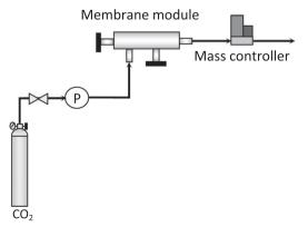
Fig. 1. Experimental setup for gas permeability testing.
