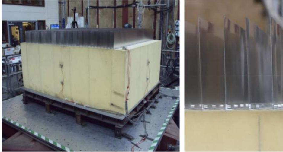
**Fig. 9** Left: shaking table (Bristol Laboratory for Advanced Dynamics Engineering) equipped with aluminum sheets acting as resonators as studied in Ref. [277]; right: zoom on the sheets (original pictures by Professor Claude Boutin)
