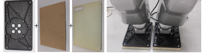
Fig. 7: Photo of HRP-2's feet with flexible soles
