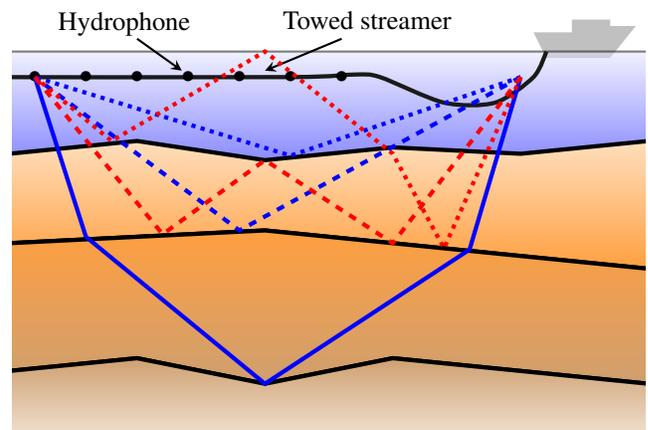
**Fig. 1.** Principles of marine seismic data acquisition and wave propagation. Towed streamer with hydrophones. Reflections on different layers (primaries in blue), and reverberated disturbances (multiple in dotted and dashed red).
