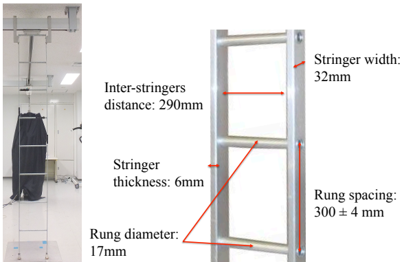
Fig. 12 The vertical ladder (left) and its parameters (right) used in HRP-2 climbing experiments. It comprises eight rungs in total and is fixed between the robot security gantry crane holder and the ground.
