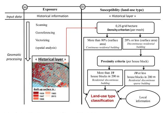
Figure 6. Evolution of vulnerability: (a) exposure and (b) susceptibility (building use type).
