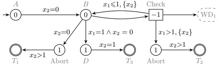
**Fig. 11.** Widget  $W_2^{=0}$ . Note that if the delay in Check is  $> 0$  then Player 1 will go to Abort and reach a target with cost = 1. Widget  $WD_1$  is the same as in the decrement module. Delay at  $B$  is  $k = \frac{4 \times 5^i}{5^{c_1} 7^{c_2}} + \varepsilon$ . If  $\varepsilon \neq 0$  then Player 2 will enter the widget  $WD_1$  and the target in  $WD_1$  is reached with cost  $\neq 1$ .
