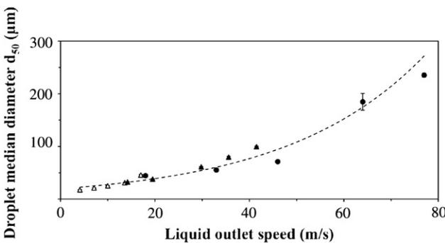
Fig. 10. Influence of liquid outlet speed on droplet diameter ( $d_{50}$ ) after atomization of pure water using three different two-fluid nozzles, at  $0.41 \text{ mm}$  ( $\Delta$ ), at  $0.46 \text{ mm}$  ( $\blacktriangle$ ), or at  $0.51 \text{ mm}$  ( $\bullet$ ) inside diameters, for an atomizing relative air pressure of  $1.5 \text{ bar}$ .
