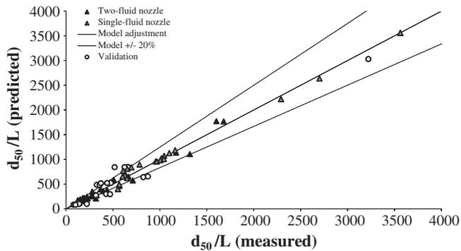
**Fig. 13.** Predicted versus experimental dimensionless droplet diameters for the single- (gray triangles) and the two-fluid (black triangles) nozzles. The droplet size measurement was carried out with a laser beam placed at a fixed distance  $L = 14$  cm from the extremity of the nozzle. Validation points of the model are shown in white circles.
