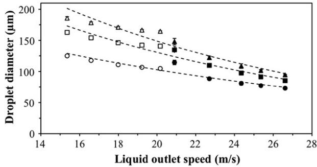
Fig. 5. Influence of liquid outlet speed on droplet diameters ( $d_{32}$  (○),  $d_{50}$  (□), and  $d_{43}$  (△)) after atomization of pure water using two different single-fluid nozzles, at 0.28 mm (white symbols) or at 0.66 mm (black symbols) inside diameters.
