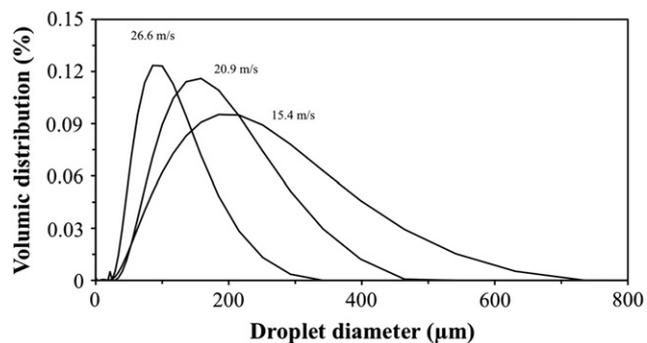
**Fig. 4.** Droplet size distributions after atomization of pure water using single-fluid nozzles of 0.66 mm inside diameter at outlet liquid speed of 26.6 m/s and 20.9 m/s, and 0.28 mm inside diameter at outlet liquid speed of 15.4 m/s.
