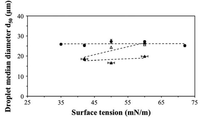
Fig. 11. Influence of liquid surface tension on droplet diameter ( $d_{50}$ ) after atomization of liquids of different viscosities ( $1 \text{ mPa.s}$  ( $\Delta$ ),  $127 \text{ mPa.s}$  ( $\blacktriangle$ ), and  $259 \text{ mPa.s}$  ( $\bullet$ )) using a two-fluid nozzle ( $0.41 \text{ mm}$  inside diameter) at  $10 \text{ m.s}^{-1}$  and a relative air pressure of  $1.5 \text{ bar}$ .
