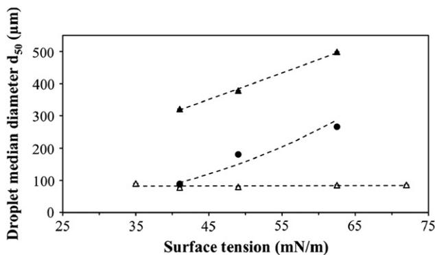
Fig. 6. Influence of liquid surface tension on droplet diameter ( $d_{50}$ ) after atomization of liquids of different viscosities (1 mPa.s (△), 25 mPa.s (●), and 72 mPa.s (▲)) using a single-fluid nozzle (0.66 mm inside diameter) at liquid outlet speed of 26.6 m.s<sup>-1</sup>.
