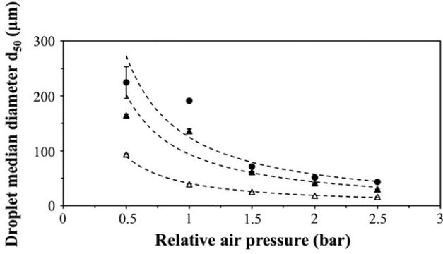
Fig. 9. Influence of relative air pressure on droplet diameter ( $d_{50}$ ) after atomization of pure water at  $10 \text{ m.s}^{-1}$  using three different two-fluid nozzles, at  $0.41 \text{ mm}$  ( $\Delta$ ), at  $0.46 \text{ mm}$  ( $\blacktriangle$ ), or at  $0.51 \text{ mm}$  ( $\bullet$ ) inside diameters.
