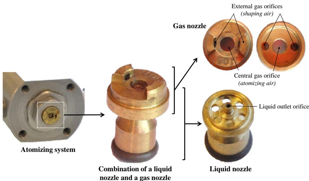
Fig. 2. Pictures of the external two-fluid atomization equipment (Spraying Systems Co., France). The gas outlet area ( $S_G$ ) corresponds to the inner area of the central gas outlet minus the outer area of the liquid outlet.
