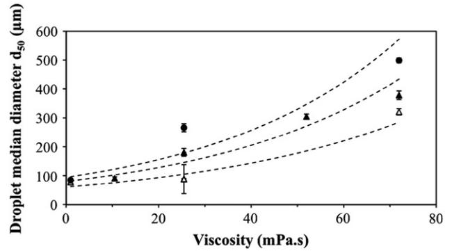
Fig. 7. Influence of liquid viscosity on droplet diameter ( $d_{50}$ ) after atomization of liquids of different surface tensions (42 mN.m<sup>-1</sup> (△), 49 mN.m<sup>-1</sup> (▲), and 62.5 mN.m<sup>-1</sup> (●)) using a single-fluid nozzle (0.66 mm inside diameter) at liquid outlet speed of 26.6 m.s<sup>-1</sup>.
