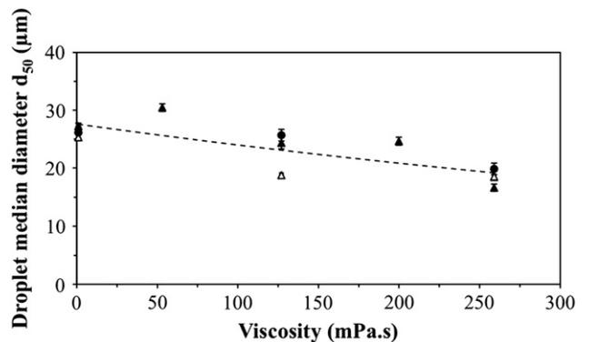
Fig. 12. Influence of liquid viscosity on droplet diameter ( $d_{50}$ ) after atomization of liquids of different surface tensions ( $42 \text{ mN.m}^{-1}$  ( $\Delta$ ),  $49 \text{ mN.m}^{-1}$  ( $\blacktriangle$ ), and  $62.5 \text{ mN.m}^{-1}$  ( $\bullet$ )) using a two-fluid nozzle ( $0.41 \text{ mm}$  inside diameter) at  $10 \text{ m.s}^{-1}$  and a relative air pressure of  $1.5 \text{ bar}$ .
