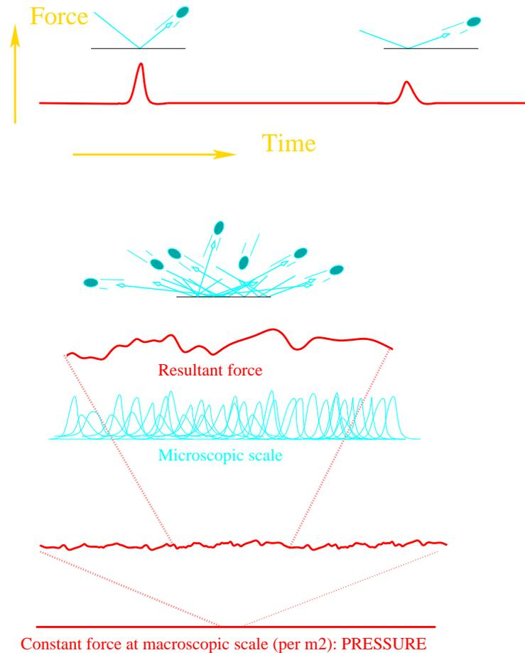
Figure 7: The device in figure 6 is used to measure the force on the plate when the number of molecules is increased. The more numerous the molecules, the more hits per unit of time and the less fluctuating the force is. At macroscopic scales, no fluctuations of the force can be detected and this constant average force per unit of surface is a stable quantity independent on the microscopic events: thus emerges the pressure.
