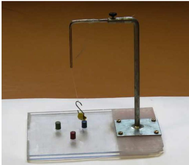
Figure 1: The magnetic pendulum is made of a magnet attracted by three other identical magnets, distinguished by a colour, which are fixed at the vertices of an equilateral triangle (here, one edge is 6 cm long). The constant length of the thread is chosen in order to avoid any contact between the magnets during the motion. This photography shows the stable equilibrium point  $M_3$  near the blue magnet.
