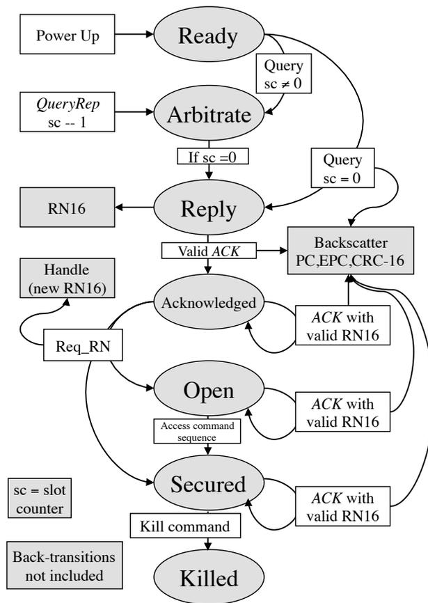
Fig. 4. EPC Gen2 tag state diagram extracted from [5]
