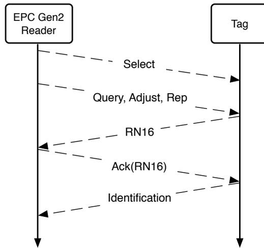
Fig. 3. Example of *Select* and *Inventory* process
