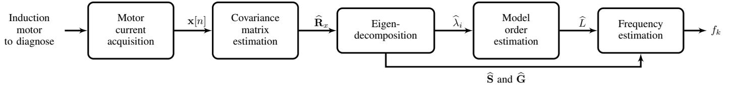
Fig. 1. Frequency estimation by using subspace techniques.
