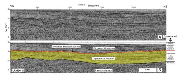
Fig. 3. Interpreted and uninterpreted seismic profile LRM96-11 across the Gulf of Lions tied to Tramontane-1 well. The erosional surface observed offshore Roussillon truncates Upper Miocene sediments and is covered by sediments from the earliest stage of the Pliocene (Cravatte et al., 1974; Guennoc et al., 2000) supporting the hypothesis that this unconformity corresponds to the Messinian Erosional Surface. The location of the seismic profile is shown in Figure 1.
