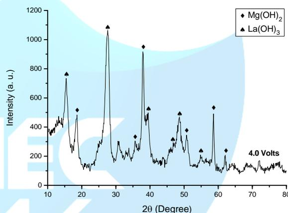
Fig. 3. X-ray diffraction pattern of the sample
