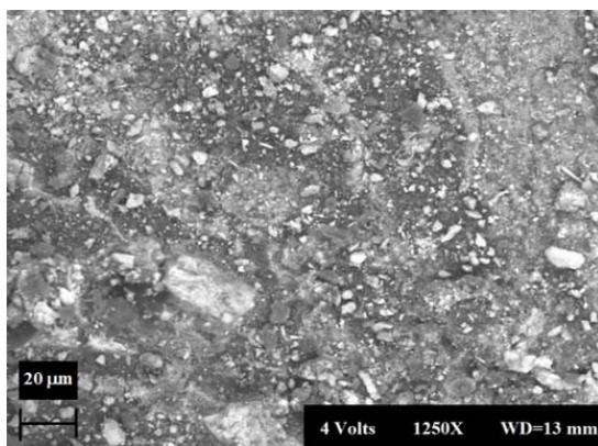
Fig. 2. SEM image of the as-deposited powder
