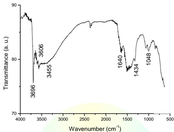
Fig. 4. FTIR transmittance spectrum of the as-prepared powder
