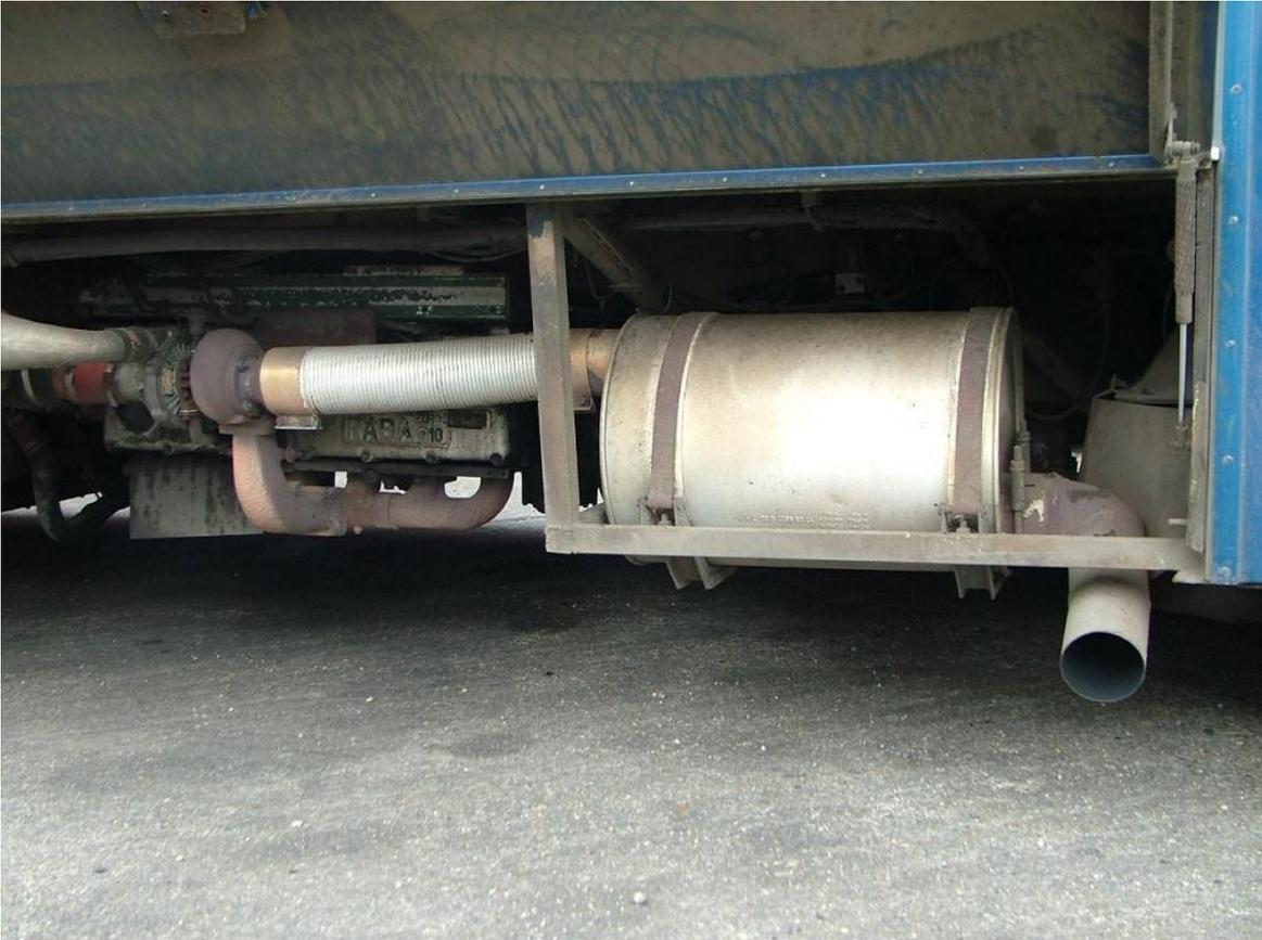
Figure 3: Rába D10UTSLL160 diesel engine with the original silencer in a bus of Ikarus 280.40 type
