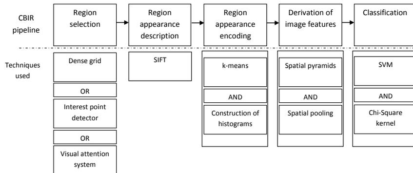
Fig. 1. pipeline of content based image retrieval algorithm
