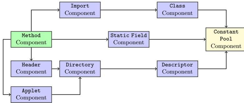
Fig. 4: Order of generation of CAP file components.
