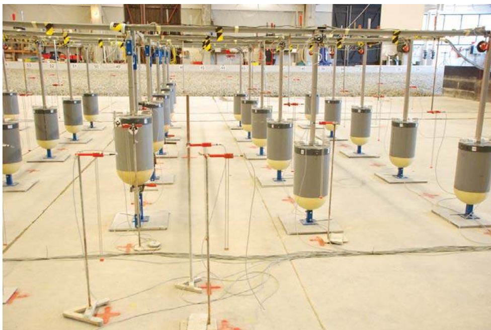
FIG. 3. The support structures for the WEC arrays.
