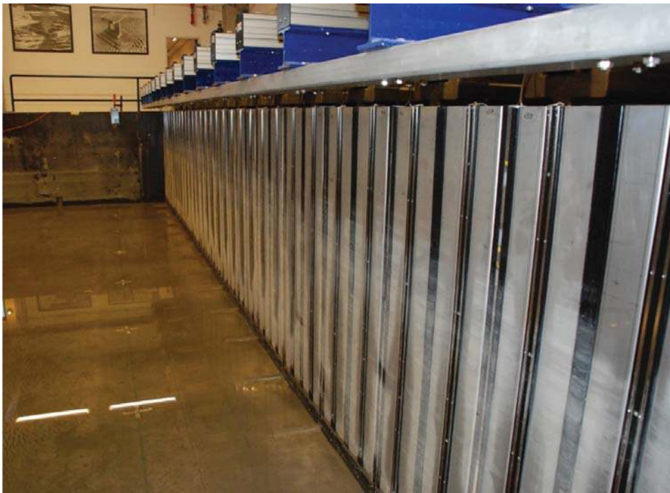
FIG. 2. Wave generator at the Shallow Water Wave Basin of DHI (Hørsholm, Denmark). View to the wave paddles from the side of the wave basin.
