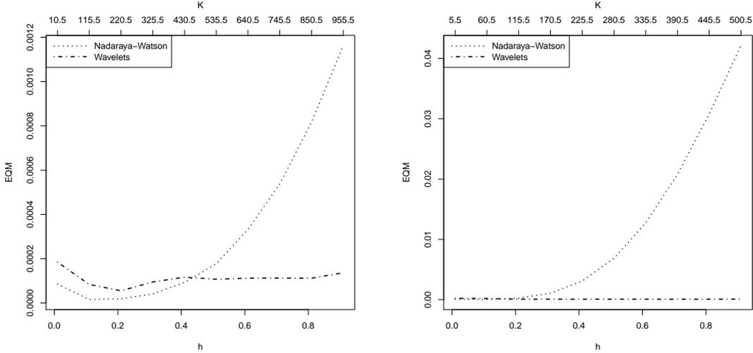
Figure 2: MSE for the estimators using Nadaraya-Watson (dots) and wavelets (dash-dots) in the case of the stochastic Ishigami model (Case 2) for  $n = 10,000$ : for  $X_1$  (left) and  $X_2$  (right). The MSE with Nadaraya-Watson estimators are plotted as functions of the window  $h$  (bottom axis) and the MSE with wavelets are plotted as function of the constant  $K$  (top axis).
