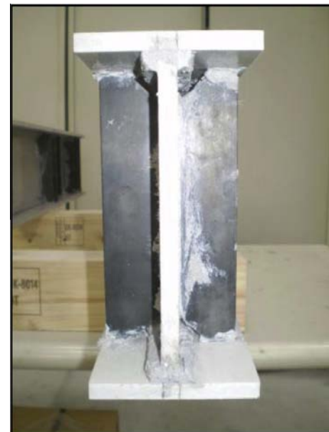
Fig. 4a. Web-flange reinforcement – cross end view.
