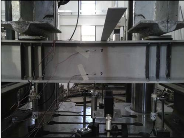
Fig. 4b. Web-flange reinforcement – frontal view.
