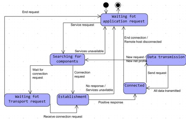
Figure 3: Description of the Transport layer behavior
