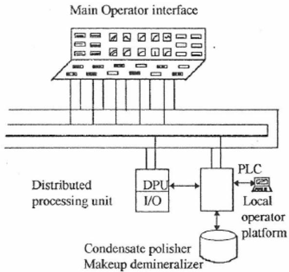
Fig. 4 - PLC Control and Local Operator Interface
