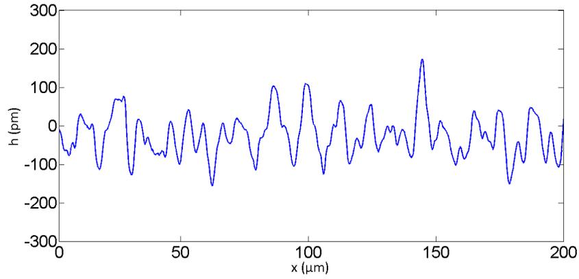
Fig. 5. Differential profile obtained on the inner surface of a silica capillary tube over a length of 200  $\mu\text{m}$ . Height fluctuations are extremely low, in the range of a few hundreds of picometers.
