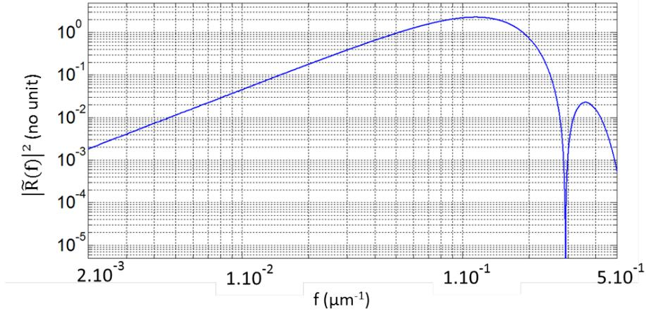
Fig. 3. Response function  $|\tilde{R}(f)|^2$  for a beam waist  $w = 1.3\mu\text{m}$  and a beam separation  $d = 3.4\mu\text{m}$ . At low frequency, the profilometer acts as a differential operator and we get the parabolic behavior  $|\tilde{R}(f)|^2 \propto f^2$ . In addition to the diffraction effect at high frequency, the zero induced by the differential operator is clearly visible at frequency  $f_d = 1/d = 0.29\mu\text{m}^{-1}$ , and can provide an experimental determination of  $d$ .
