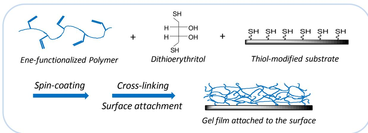
**Figure 1.** Schematic of hydrogel films synthesis: ene-reactive polymer is spin-coated on thiol-modified substrate with dithiol crosslinkers. Thiol-ene click reaction allows simultaneous polymer chains crosslinking and surface attachment.
