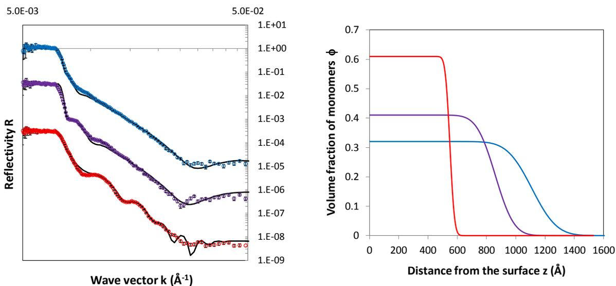
**Figure 5.** (Left) Neutron reflectivity curves of PNIPAM hydrogel film (with dry thickness equal to 36.4 nm) in water at three temperatures 25°C, 34°C and 40°C. Also are shown the best fitting of the experimental data. Circles are for data and lines for fitting. (Right) Volume fraction profiles corresponding to the best fitting. The same color code as the left figure with reflectivity curves is used: blue for 25°C, purple for 34°C and red for 40°C.
