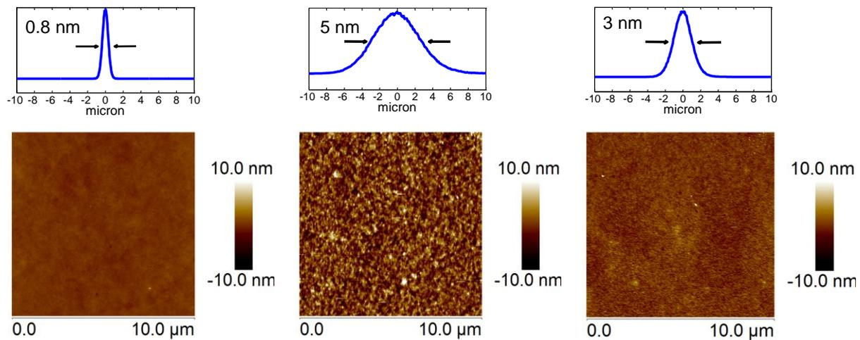
**Figure 6.** Height AFM images of PNIPAM hydrogel films in air (left), in water at 25°C (middle) and in water at 40°C (right). Images are obtained in air with tapping mode and in water by using QNM mode with a cantilever of stiffness 0.02 N/m. The thickness of PNIPAM hydrogel film is 250 nm in air, it is equal to 960 nm in water at 25°C and 360 nm at 40°C. The corresponding height histogram is displayed on the top. Roughness is determined from the half width of the peak.
