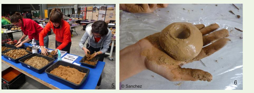
Wetness is very important, the earth has to be wet enough, but not too much to be compacted without sticking, and to avoid breaks when drying (archi.1)
