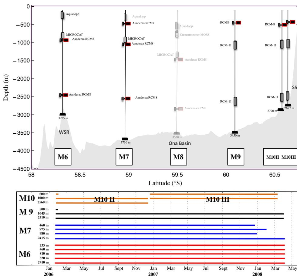
**Figure 3.** (top) Distribution of the mooring lines and instruments. Mooring M8 (half-toned) was lost. The South Scotia Ridge (SSR) and West Scotia Ridge (WSR) are labeled. (bottom) measurement calendar.
