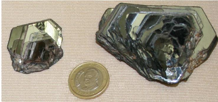
Figure 2. Rose-shaped hematite crystal with reflecting metallic gray aspect on the largest platelets and red appearance along the thickness. The latter is close to the deeply red streak of this material.
