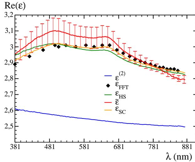
Figure 8. Real part of the complex permittivity  $\tilde{\epsilon}$  of the hematite coating: Hashin and Shtrikman estimate (green), self consistent estimate (orange), ellipsometry measurements (red) and numerical FFT predictions (black symbols). Blue, for comparison: ellipsometry measurements of the real part of the complex permittivity of the epoxy.
