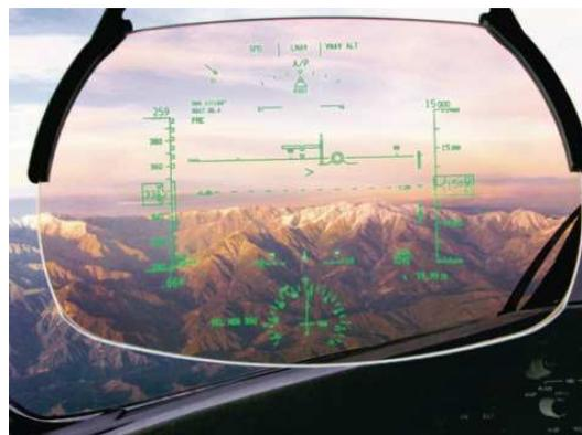
**Fig. 3.** Close-up view of the Boeing 787 head up display
