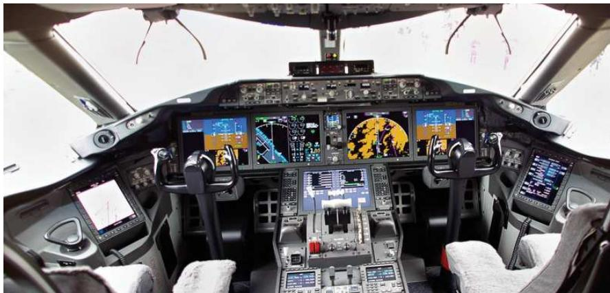
**Fig. 2.** The Interactive Cockpit of new Civil Aircrafts (here Boeing 787)
