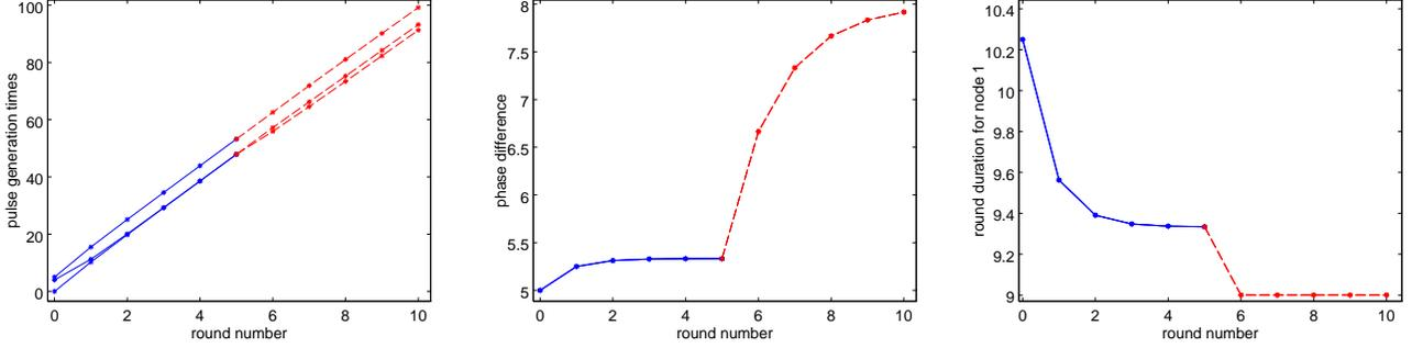
Fig. 3. Prefix of an execution of the example dynamic network for rounds  $0 \leq k \leq 10$ . The communication graph changes from  $G_1$  (solid lines) to  $G_2$  (dotted lines) at round 5. The figure shows (i) pulse generation times  $t_i(k)$ , (ii) maximum phase differences  $\max_{i,j} |t_i(k) - t_j(k)|$ , and (iii) round durations  $t_1(k+1) - t_1(k)$ .
