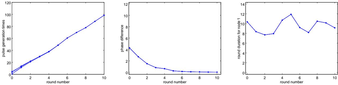
Fig. 6. Prefix of an execution of the example dynamic network of size  $n = 5$  for rounds  $0 \leq k \leq 10$ . Communication graph  $G(k)$  are directed random graphs, with probability 0.6 of a link to be in  $G(k)$ . We run the fixed weight algorithm with parameter  $c = 1/10$ .
