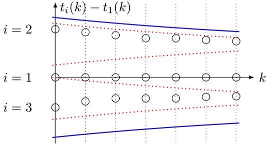
Fig. 5. Phase differences of three nodes to node 1 over rounds  $k$  in stable environments. The outer solid hull follows from Theorem 5. The inner dotted hulls follow from Theorem 10, showing that phase differences cannot vary arbitrarily within the outer hull.
