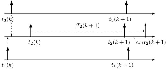
Fig. 1. Round  $k$  and  $k+1$  pulses of a three node system. Node 2 adapts the time of occurrence of its round  $k+1$  pulse by a negative offset  $\text{corr}_2(k+1)$  due to the early pulses received from nodes 1 and 3.
