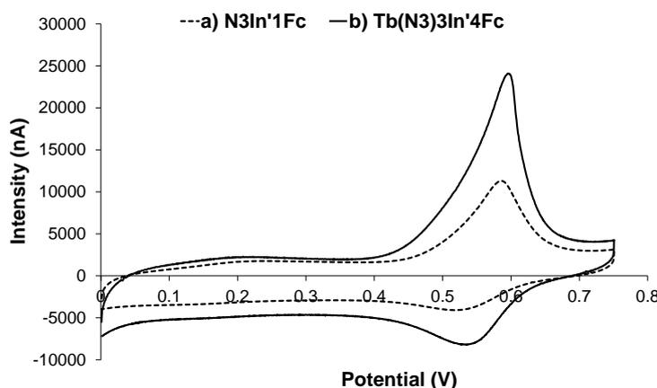
**Fig.4.** Cyclic voltammograms recorded on a gold electrode functionalized with a)  $N_3In'1Fc$ ; b)  $Tb(N_3)_3In'4Fc$  (scan rate of  $0.1 \text{ V s}^{-1}$  *vs.* SCE)
