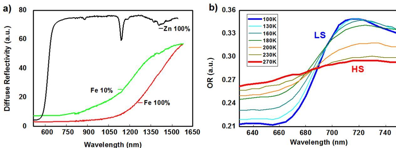
**FIG. 2.** **a)** diffuse reflectivity spectra collected on powders of  $[\text{Fe}(\text{PM-AzA})_2(\text{NCS})_2]$  (—),  $[\text{Zn}_{0.9}\text{Fe}_{0.1}(\text{PM-AzA})_2(\text{NCS})_2]$  (—) and  $[\text{Zn}(\text{PM-AzA})_2(\text{NCS})_2]$  (—) crystals. **b)** optical reflectivity spectra of a  $[\text{Fe}(\text{PM-AzA})_2(\text{NCS})_2]$  single crystal acquired at different temperatures during the SCO from pure LS (100 K) and HS (270 K) states.
