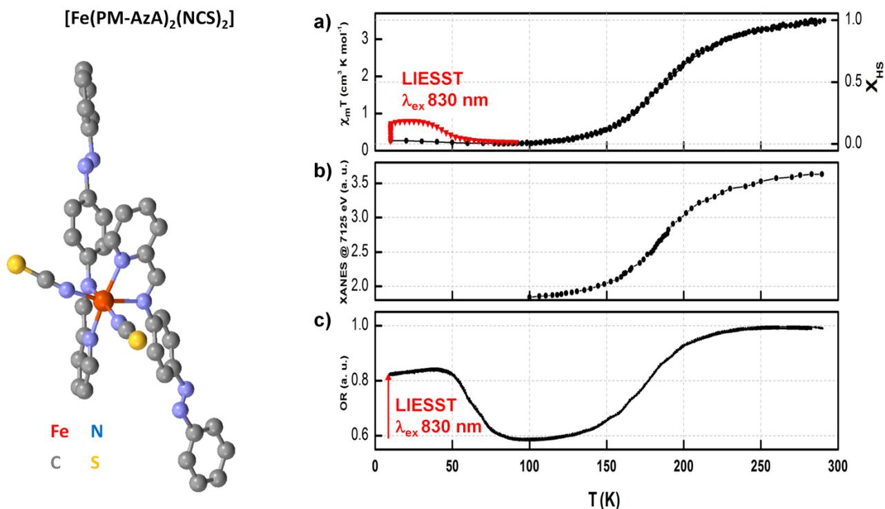
**FIG. 1.** Thermal spin crossover of the [Fe(PM-AzA)<sub>2</sub>(NCS)<sub>2</sub>] compound (top) monitored with the evolution of **a)**  $\chi_M.T$  product, **b)** X-ray absorption at 7125 eV, **c)** total optical reflectivity. The increase of  $\chi_M.T$  and OR under cw light excitation at 830 nm in a) and c) is related to the long-lived LIESST phenomenon at low temperature.
