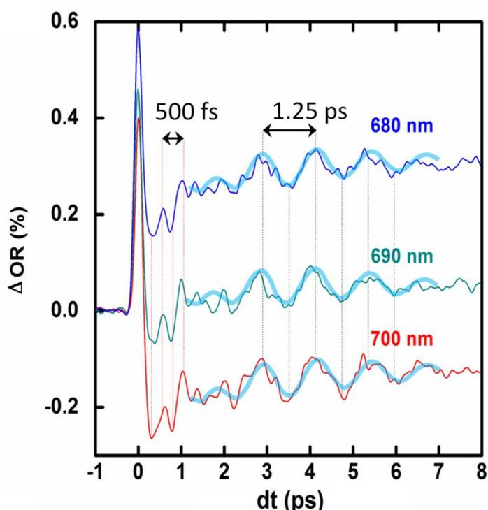
**FIG. 6.** Dynamical OR time traces recorded at 680 nm, 690 nm and 700 nm after photoexcitation at 800 nm ( $0.4\text{ mJ/mm}^2$ ) and showing in phase oscillations of the reflectivity signal. Thick cyan curves represent the fit to the data with a sine function multiplied with an increasing and decreasing exponential terms.
