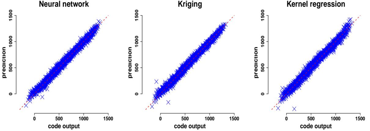
Figure 3: Plot of the metamodel predictions in the test base (y-axis), as a function of the Germinal output values (x-axis), for the neural networks (left), Kriging (middle) and kernel methods (right). Case of the original computations. The dashed lines is defined by  $y = x$ .
