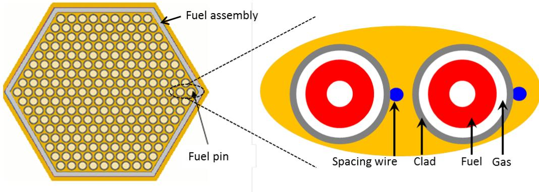
Figure 2: A schematic representation of a fuel pin and a fuel assembly in nuclear fast-neutron reactors.
