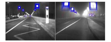
Fig. 8. Illustration of source halos' detection. (Left) Without fog. (Right) With fog. Expanding blue boxes represent the bounding boxes of the connected components at each step.
