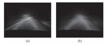
Fig. 5. Video sequence grabbed in actual fog during a test drive. (a) Sample frame. (b) Mean of successive frames. The objects in the scene are suppressed, whereas the backscattered veil remains due to its temporal stability.
