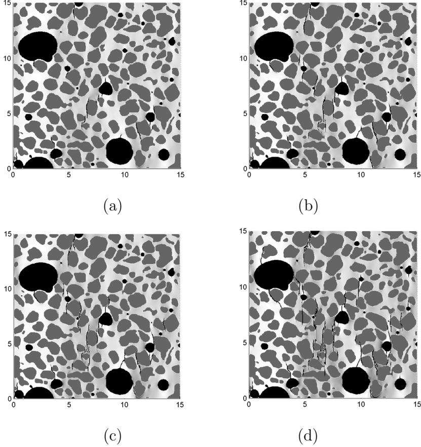
Fig. 31. Compression test on a microtomography image-based model of EPS lightweight concrete: microcracking evolution for:  $u_a = 0.12$  mm,  $u_b = 0.15$  mm,  $u_c = 0.162$  mm and  $u_d = 0.18$  mm (see Fig. 32 for corresponding force-displacement curve).
