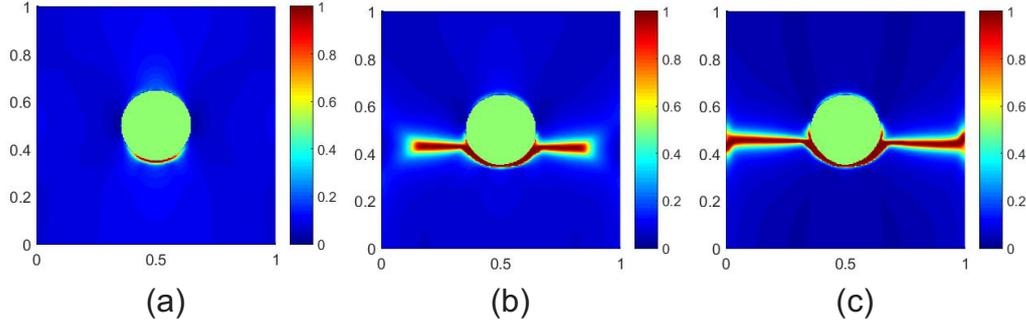
Fig. 22. Crack paths obtained with different length parameter  $l_\beta$  for the same load  $\bar{U} = 0.0107$  mm: (a)  $l_d/l_\beta = 1/3$ ; (b)  $l_d/l_\beta = 1$ ;  $l_d/l_\beta = 2$ ,  $l = 0.013$  mm.
