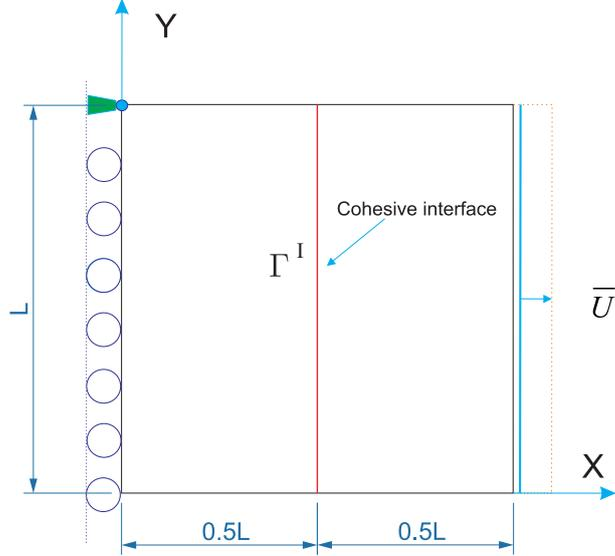
Fig. 6. Discontinuous benchmark, geometry and boundary conditions.
