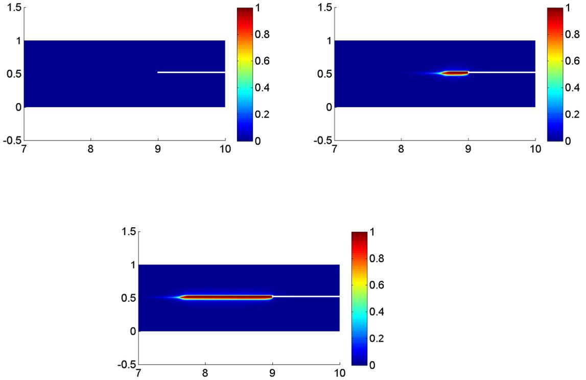
Fig. 17. Delamination peel test problem: phase field evolution  $d(\mathbf{x})$  for:  $u = 0$  mm,  $u = 0.4$  mm and  $u = 1$ mm
