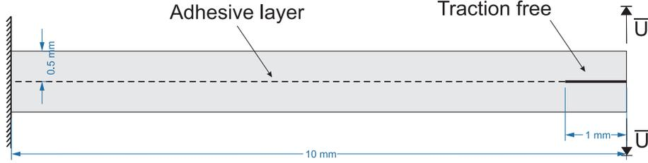
Fig. 16. Delamination peel test problem: geometry and boundary conditions
