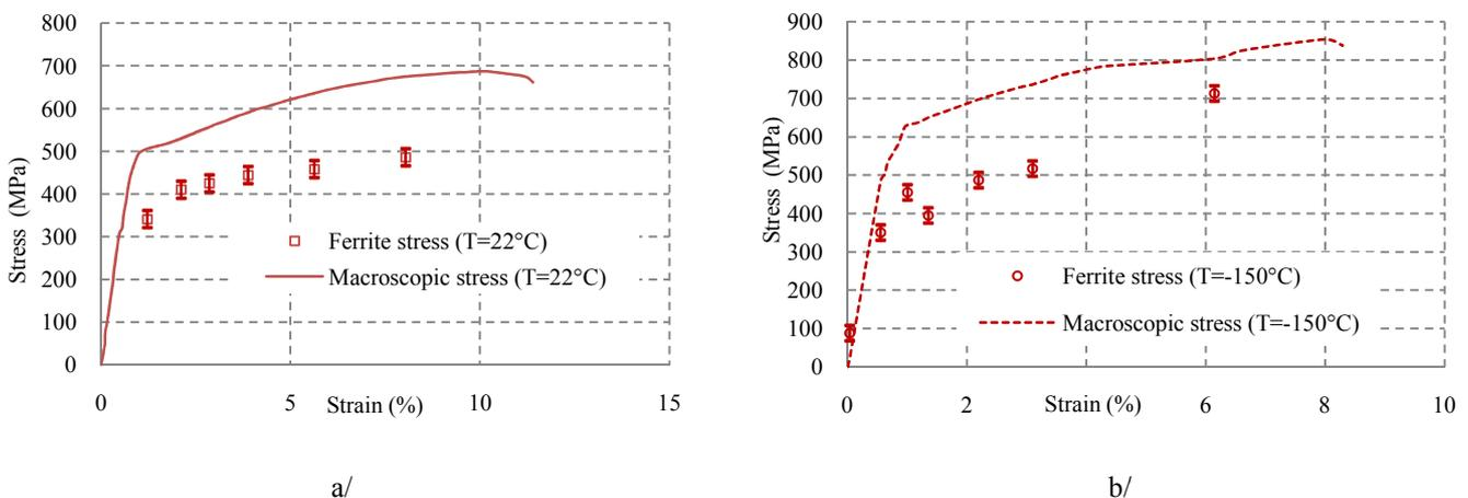
**Fig. 4: Stress evolution in ferrite phase, 16MND5 steel - a/  $T=22^{\circ}\text{C}$  - b/  $T=-150^{\circ}\text{C}$**
