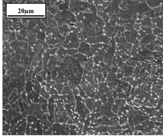
**Fig. 2: SEM micrograph showing the microstructure of the XC40 steel**
