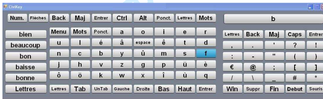
36 37 Figure 3: CVK dynamic on-screen keyboard with word prediction list on the left
